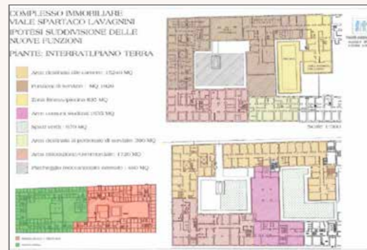
3) Floor plans of level types with a hypothesis for the distribution of new features
